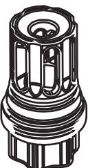
The Pursuit Series features a shrouded, vented end cap that promotes consistent gas flow, further refining the recoil impulse and enhancing overall suppressor performance.
