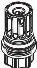
The Pursuit Series features a shrouded, vented end cap that promotes consistent gas flow, further refining the recoil impulse and enhancing overall suppressor performance.
